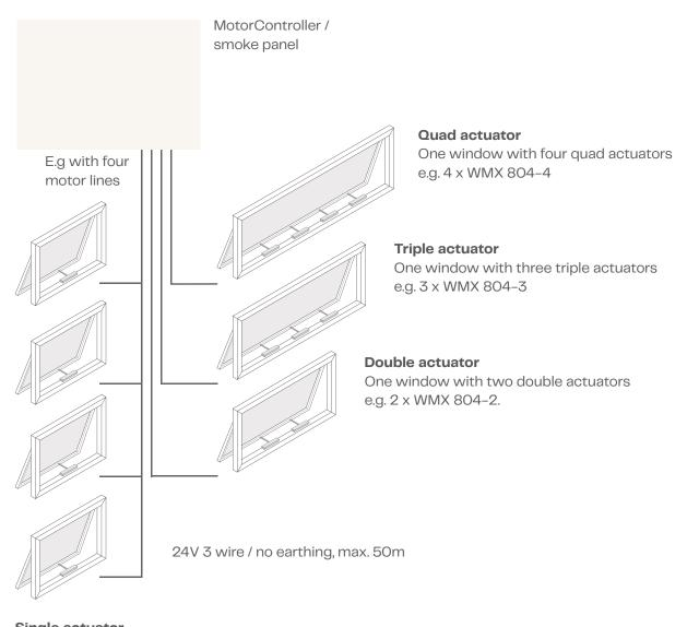
Single actuator One window with one single actuator e.g. 1 x WMX 804–1. Up to four windows each with one actuator e.g. 4 x WMX 804–1 can be connected.)
